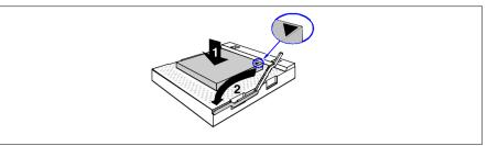
Figure 9: Installing the processor
